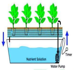
**6. Ebb and flow technology:** It is also known as "flood and drain hydroponics". According this system, plants are grown in a soil-less medium and periodically flooded with a nutrient- enriched water solution by using a pump that is placed into the reservoir and allowing it to drain back into the reservoir. It supplies oxygen to roots, and it helps to prevent overwatering.
