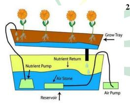
. Nutrient film technique: It was developed by Dr. Allen Cooper in England in the 1960s. In this system, a thin layer of nutrient solution constantly flows over the roots of the plants in a shallow, sloping channel (Morgan, 2009). There is a small amount of water around the roots of the plants, which is the main reason for naming this method NFT.
